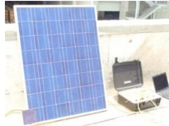
Spectral response testing
